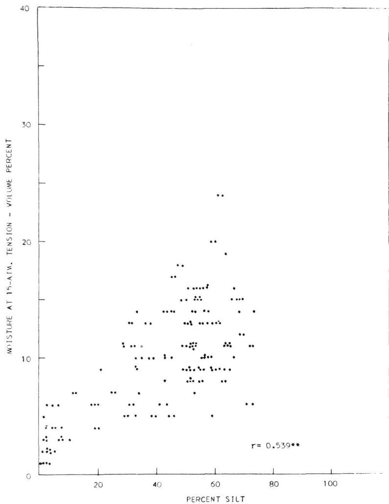
Figure 5. 15-atm. percentage as a function of silt content.
