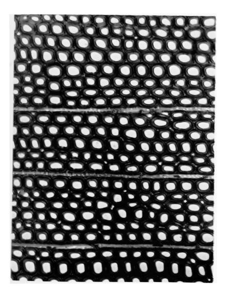
Figure 10. Azure B, showing possible lignin distribution across the mature secondary wall. Higher lignin content, dark greenish-blue; lower lignin content, light green. Section of FAA-killed and celloidin embedded compression wood sample collected June 21, 1966; X 2000.
