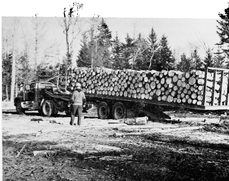
Figure 2. A loaded pallet in final stages of being winched aboard a pallet truck.
