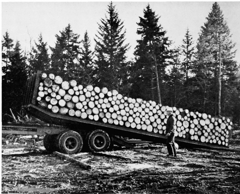
Figure 1. A loaded pallet in initial stages of being winched aboard a pallet truck.
